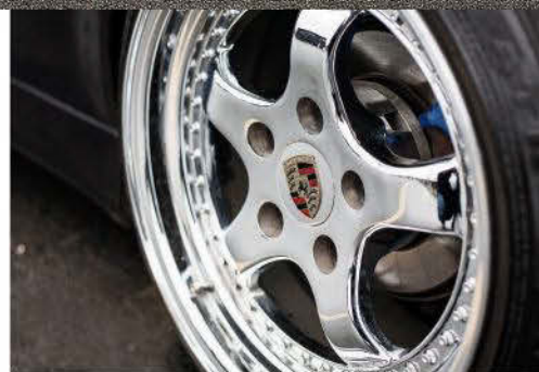
Custom 17" BW Motorsports wheels use OEM Porsche centers and Kinesis rims
