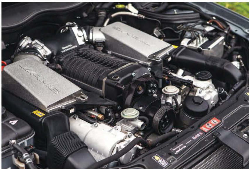
Weistec stage 2 supercharger conversion increases output from 500 to 672hp
