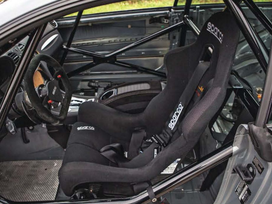
Stainless steel cage meets NASA regulations and includes aluminum driver protection zone
